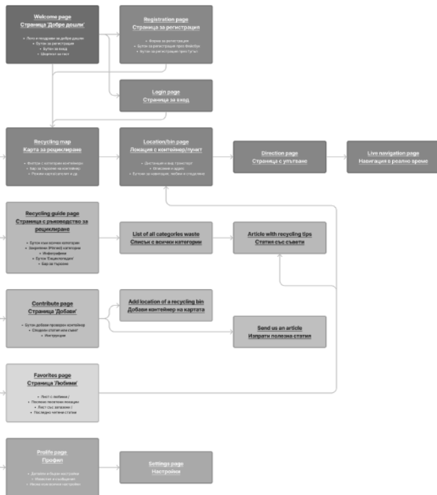
Fig. 3. Structure diagram of App [Students works in Usability Engineering, 2023]
