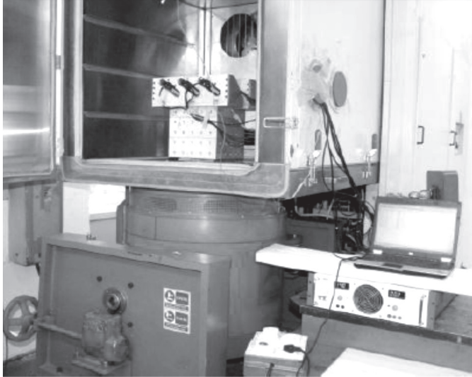
Fig.2. Example of vibrational test bench
