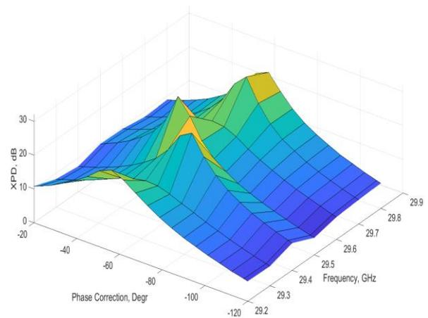
Fig. 7. Phase tuning. Measurement data. Surface representation
