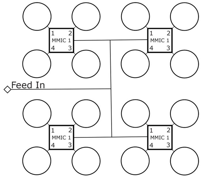
Fig. 3. Simplified antenna layout.
