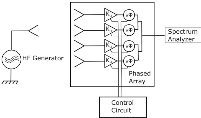
Fig. 2. Test Setup - Block Diagram.
