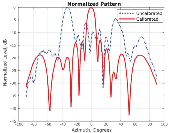
Fig. 6. Patterns before and after calibration
