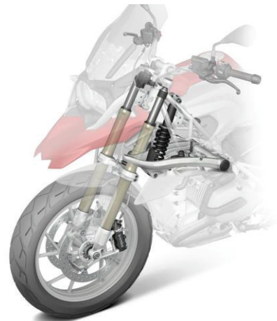
Fig. 2. Telelever suspension type. (BMW Motorrad)
