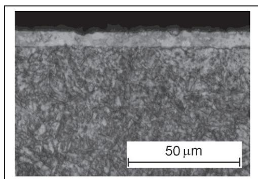
Fig. 1. Ni-coating microstructure after heat treatment at 290°C, 6h (sample 2)
