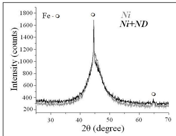
Fig. 3. X-ray diffraction pattern of samples 1 (Ni coating) and 3 (Ni/Ni+ND coating) in an as-plated condition.
