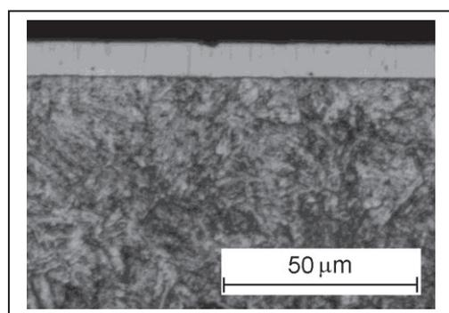
Fig. 2. Ni/Ni+ND coating microstructure after heat treatment at 290°C, 6h (sample 4)
