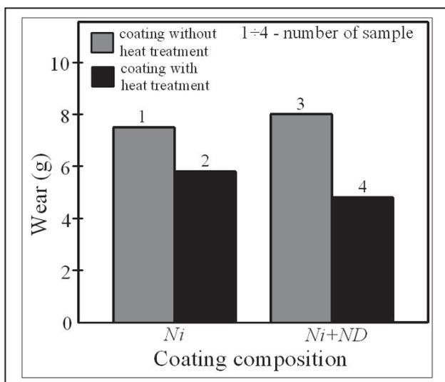
Fig. 6. Wear of the coatings Ni и Ni/Ni+ND
