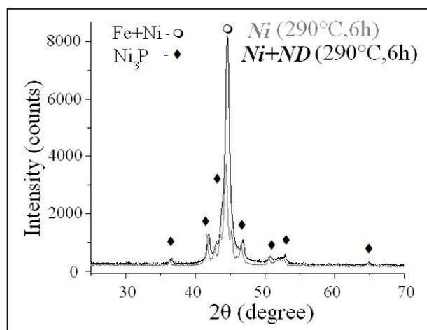
Fig. 4. X-ray diffraction pattern of samples 2 (Ni coating) and 4 (Ni/Ni+ND coating) after heat treatment at 290°C, 6h.
